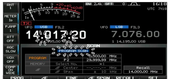
▨ If the same frequencies are programmed into the scan edge memory channel P1 and P2, programmed scan will not start.
