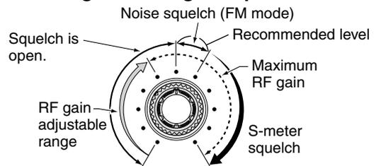
**• When functioning as an RF gain control**
