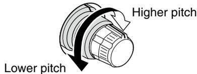
**54 MANUAL NOTCH FILTER CONTROL [NOTCH]**
