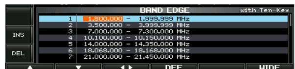
▨ **NOTE:** All frequency ranges are set in default. So you should delete or change it to add the desired band edge frequency.
