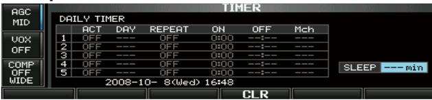
The sleep timer turns the transceiver power OFF automatically after passing the set period. The timer can be set to 5–120 min. in 5 min. steps.
