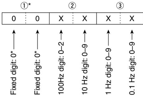
\*Not necessary when setting a frequency.
