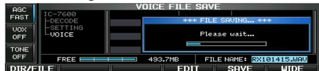
When a PC keyboard is connected to the [USB] connector on the front panel, the file name can also be edited from the keyboard. In this case, a USB hub is required.
