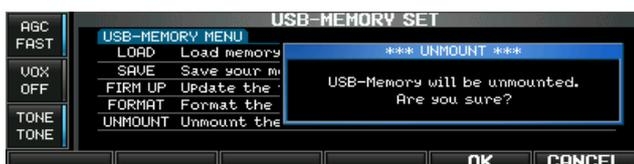
**CAUTION:** When removing the USB-Memory, unmount operation is recommended. If you do not unmount the memory, data on the USB-memory may be corrupted.
