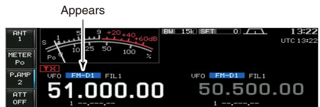
**NOTE:** When data mode is selected, the audio input from the [ACC1] (pin 4) is used for transmission instead of the [MIC]'s depending on the set mode settings. Modulation input connector can be changed in the ACC set mode (p. 124)
