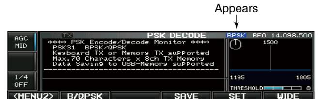
• **PSK decode screen— the QPSK mode**
