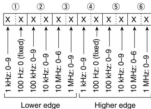
**• Data mode with filter width setting**
