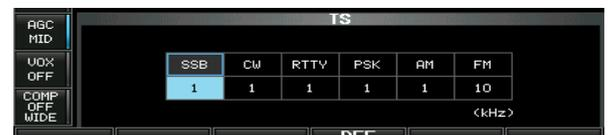
**NOTE:** When entering the quick tuning step set mode, the quick tuning function must be activated first.
