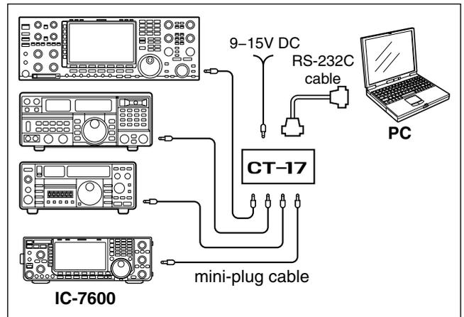
When the transceiver is connected to a PC with the USB cable (purchased separately), the optional CT-17 is not required.
