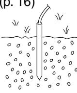
Use the heaviest gauge wire or strap available and make the connection as short as possible.
