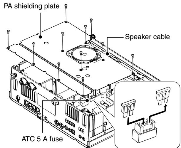
**WARNING:** DO NOT pull the speaker cable when removing or replacing the PA shielding plate. Otherwise, a fire, injury or damage the transceiver may occur.
