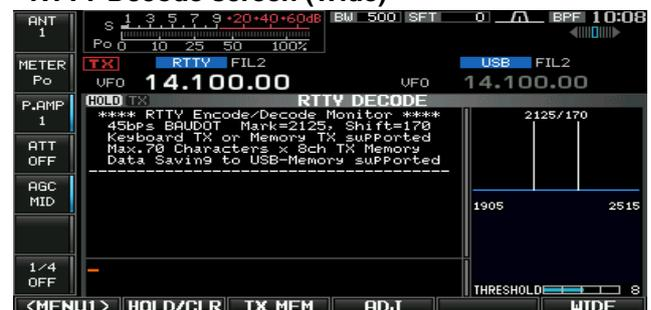
◆ **Setting the decoder threshold level**
