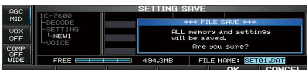
Memory channel contents, set mode settings, etc. can be saved into the USB-Memory for backup.
