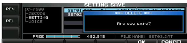
**RECOMMENDATION!** Deleting the setting file is irreversible. Confirm the contents before deleting a setting file!
