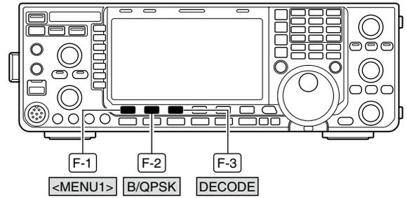
• **PSK decode screen— the BPSK mode**
