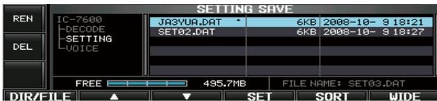
When a PC keyboard is connected to the [USB] connector on the front panel, the file name can also be edited from the keyboard. In this case, a USB hub is required.
