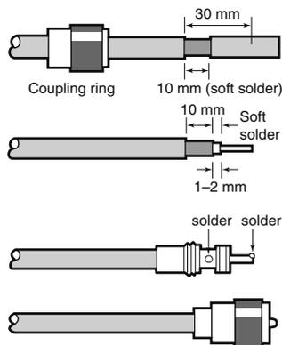
① Slide the coupling ring down. Strip the cable jacket and tin.
