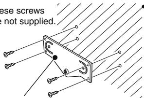
Attach the remote controller bracket onto a flat surface using 4 self-tapping screws (2.6 mm(d)), or double-sticky tape, etc., as at left, then attach remote controller to the bracket.
