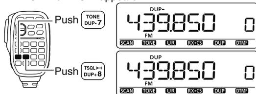
3 Push [FUNC] then [DUP- 7(TONE)] to turn ON the subaudible tone encoder according to repeater requirements.
