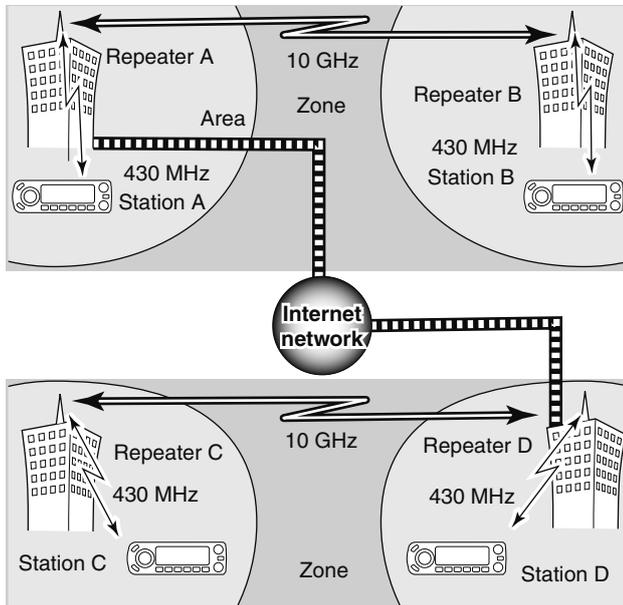
In traditional repeater operation, stations that are communicating must both be in the repeater's operating area. However, D-STAR repeaters can be linked via a 10 GHz backbone, as shown in the illustration at left. Using D-STAR, stations A and B can communicate even though they are in widely separated repeater operating areas.
