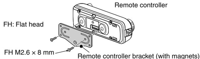
**CAUTION: NEVER** use any other than the supplied screws (FH M2.6 x 8 mm) for attaching the remote controller bracket. Otherwise the transceiver's internal board may be damaged.
