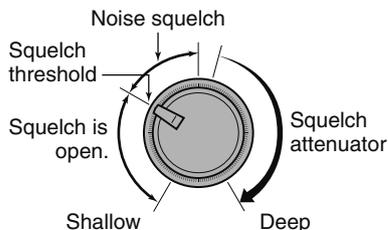
**NOTE:** The squelch attenuator functions even when the monitor function is in use. We recommend setting the **[SQL]** control between the 10 and 13 o'clock positions when using the monitor function.
