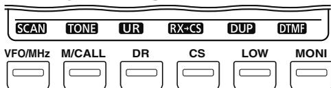
These function guides indicate the secondary functions for below the keys. Push and hold for 1 sec to activate the indicated functions. See page 2 to 3 (⑤ to ⑩).
