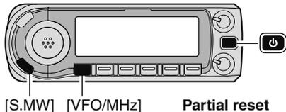
➔ While pushing and holding [S.MW] and [VFO/MHz] keys, push and hold [POWER] for 1 sec. to reset the CPU.
