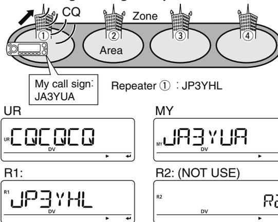
Pushing and holding **[BAND]** for 1 sec. selects the repeater group when in selection mode.
