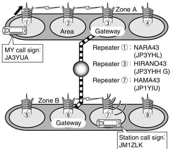
**NOTE:** If the other station has accessed the repeater at least once, the D-STAR system will connect to the repeater automatically even you don't know where the station is (possible in the same area as you, or in the same zone or a different zone). In this case, you select "GW" as the RPT2 selection. The Auto gateway setting "GW SET" is helpful (p. 136).
