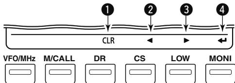
Set condition guides appear when the transceiver enters the MENU screen, select memory write state, etc.
