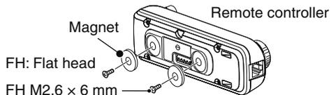
**CAUTION: NEVER** use any other than the supplied screws (FH M2.6 x 6 mm) if re-attaching the magnets to the remote controller. Otherwise the transceiver's internal board may be damaged.
