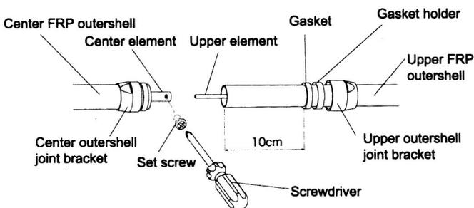
3. Connect the center and lower elements by securing set screws firmly.
