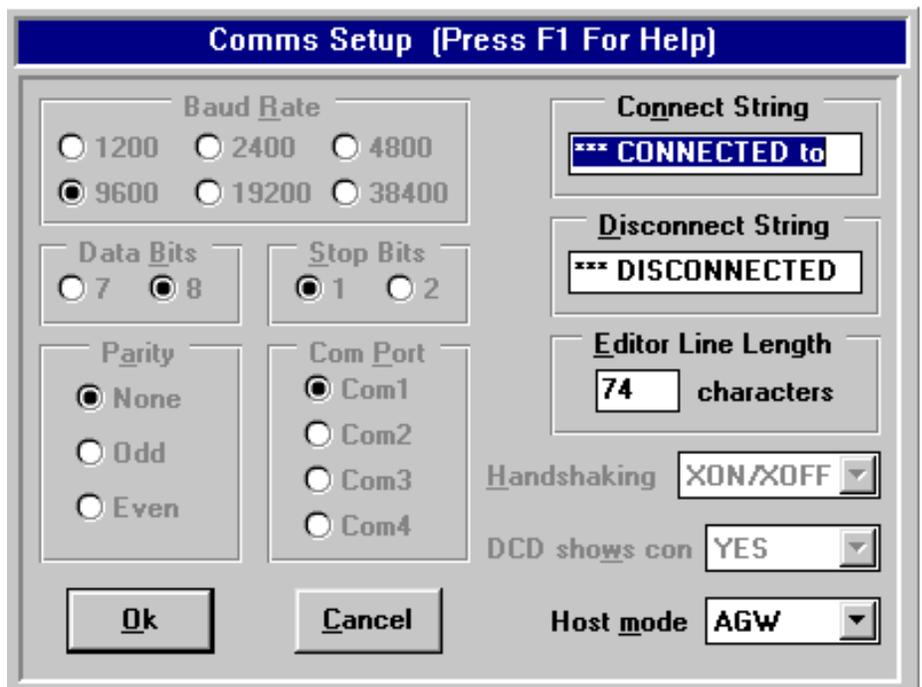
If you will be using AGWPE as your only packet input source, then you don't need to worry about setting the normal TNC parameters such as baud rate, parity, etc. AGWPE handles all that! In fact, the TNC parameters on this screen will 'gray out' (become inaccessible) since there is no need for them when you use AGWPE host mode.
