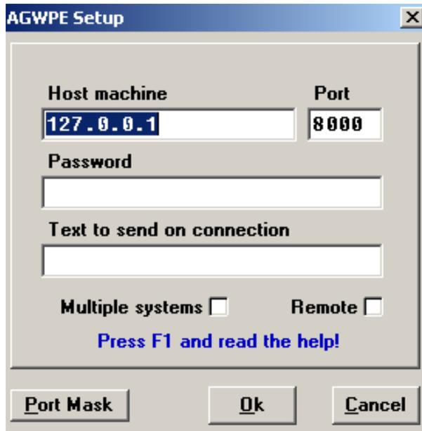
This screen is similar to the one in UI-View 16 in that you must specify the port and IP address of the computer running AGWPE. Use 127.0.0.0 (or localhost) if AGWPE is running on the same computer machine as UI-View.
