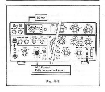
Place MODE switch to TUNE, METER switch to ALC.
