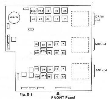
Frequency for **BAND Switch** adjustments 1.9 MHz 1.5 3.5 3.75 7.15 7 10.125 10 14 14.175 18 18.125 21 21.225 24.5 24.95 28 5 28 B
